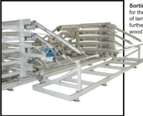
**Sorting equipment** for the optimum sorting of lamella quality before further processing of the wood
