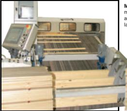
Magazine table with manual feeding and automatic extraction of lamellas
