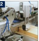
After the glue is applied, the lamellas are cross led by means of V-belt conveyors into a device where they are set-up on edge - and further on into a magazine where they are gathered. The V-belt conveyors ensure a smooth and constant cross conveying
