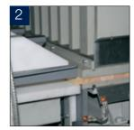
The glued lamellas are fed into the fully automatic press which consists of two parts: a high-frequency unit in front and a hot press unit behind.
