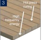
The high-frequency energy targets the liquid in the glue which quickly heats up from the inside and cures.
