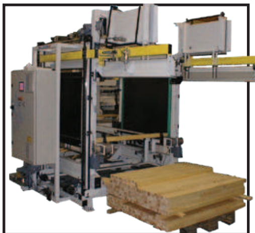
Work piece destacker for automatic destacking from pallets
