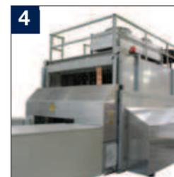
In order to optimize the production line further to an order-based production, the press can be manufactured with a semi-automatic setting of the press height enabling different products to be pressed in rapid succession, and with side pressure widths from 1280 mm and down to 240 mm, so that single or few beams can be produced by themselves according to order. Flexibility is the keyword.
