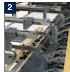
After the cross conveying, the glued lamellas are set up on edge, aligned, and joined together on a belt conveyor where they are efficiently held in place, while subsequent lamellas are added.
