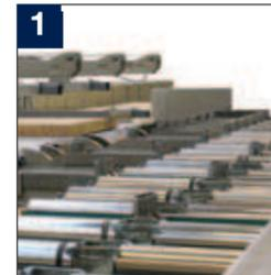
The line is fed by a high-speed dual roller conveyor, allowing the lamellas to be conveyed to the lay-up system at a quick pace. The lamellas are cross conveyed in two steps, in order to prevent collision during transport.
